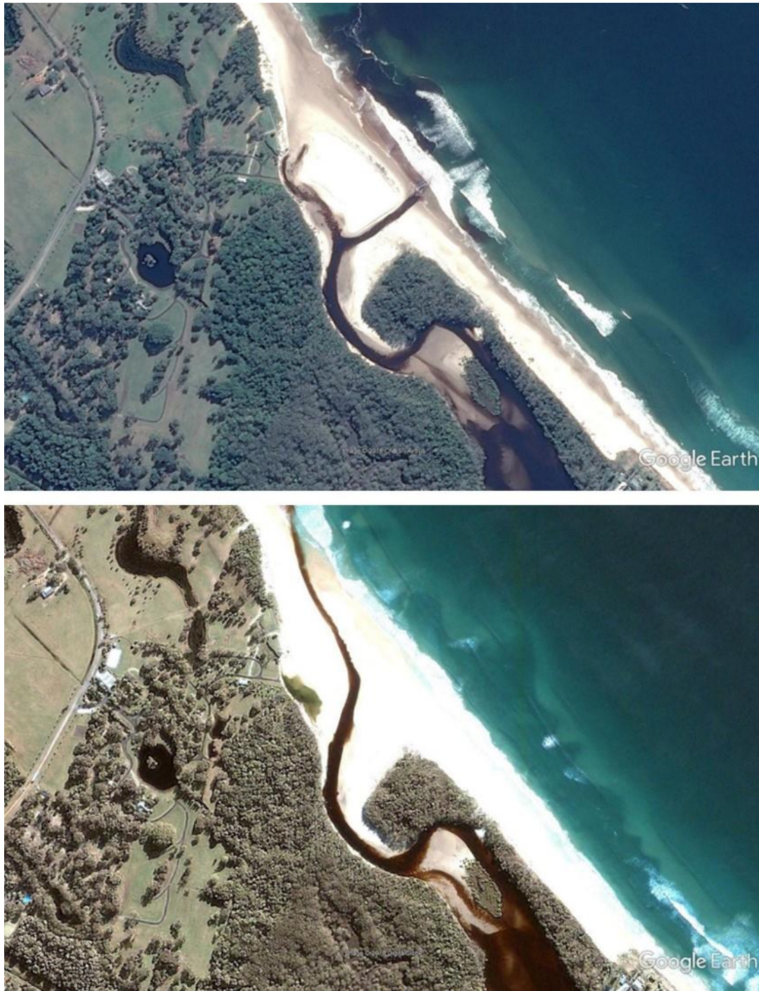
Figure 18 Comparison of Entrance Configuration on 16 May 2013 (Top) and 22 July 2013 (Bottom). The entrance was opened on 13 th May. (Source: Google Earth). Note the tendency towards northwards migration of the entrance channel driven by the dominant south to north alongshore drift.
