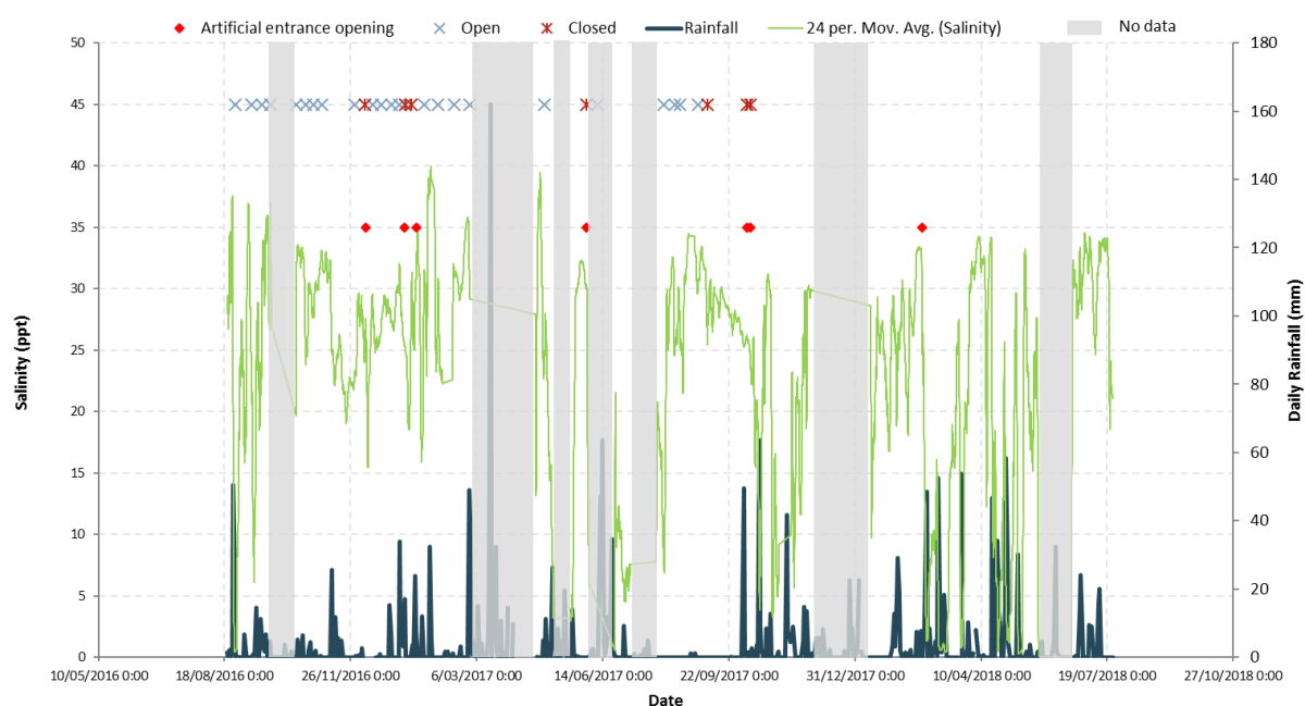
Figure 28. Moving average of salinity (data collected from HANNA multi parameter logger downstream of Ewingsdale Bridge), daily rainfall (Source:BOM) and entrance opening condition (data extracted from Council inspection sheets)
